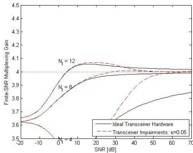
Fig.2.2 Finite-SNR multiplexing gain for an uncorrelated Rayleigh fading channel with  $N_r = 4$  and  $N_t \geq 4$ .
