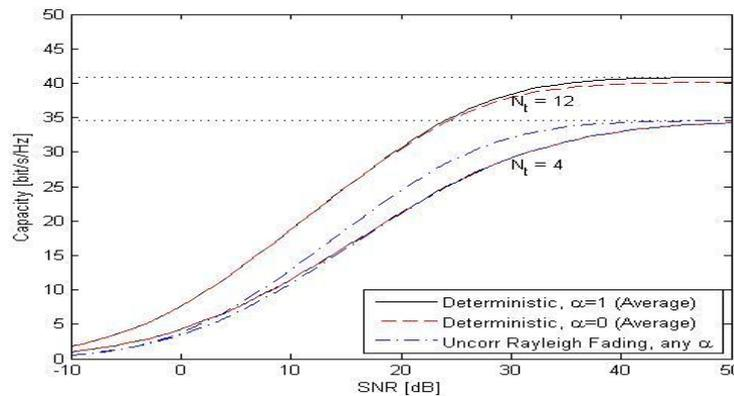
Fig.2.0 Average capacity of a 4x4 MIMO channel over different deterministic channel realizations, different levels of transceiver impairments, and  $\alpha = 1$ .
