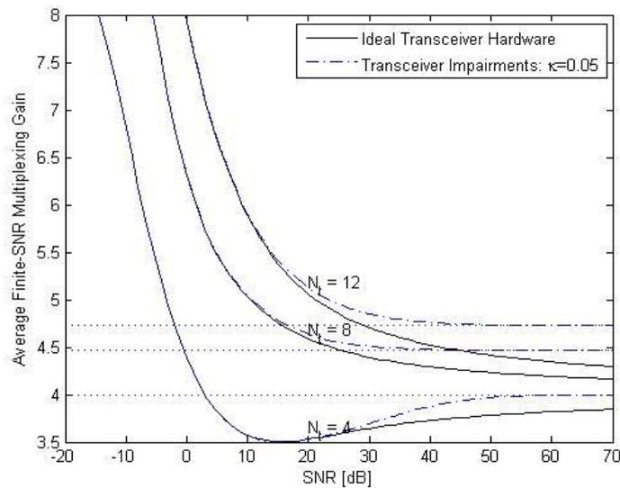
Fig.2.3 Average finite-SNR multiplexing gain of deterministic channels (generated with independent  $CN(0, 1)$ -entries) with  $N_r = 4$  and  $N_t = 4$ .
