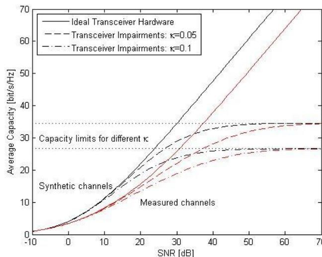
Fig.2.1 Capacity of a MIMO channel with  $N_r = 4$  and impairments with  $K = 0.05$ . We consider different  $N_t$ , channel distributions, and  $\alpha$ -values
