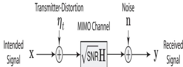
**Fig 1.0.: Block diagram of the generalized MIMO channel considered in this letter. Unlike the classical channel model, the transmitter distortion generated by physical transceiver implementations is included in the model.**
